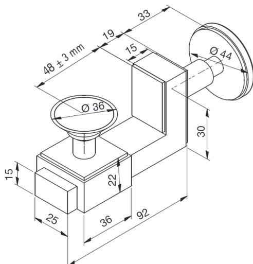
Figure 2: The connection of the stairs
